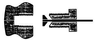
Figure 3-1. Assembling Flangless Fittings.
